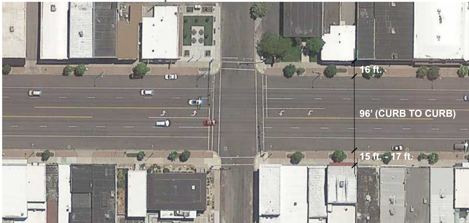
Figure 2.7 The existing sidewalks on Main Street vary slightly. The Vision Plan proposes to make them the same width and add bump outs for safety and aesthetics.
