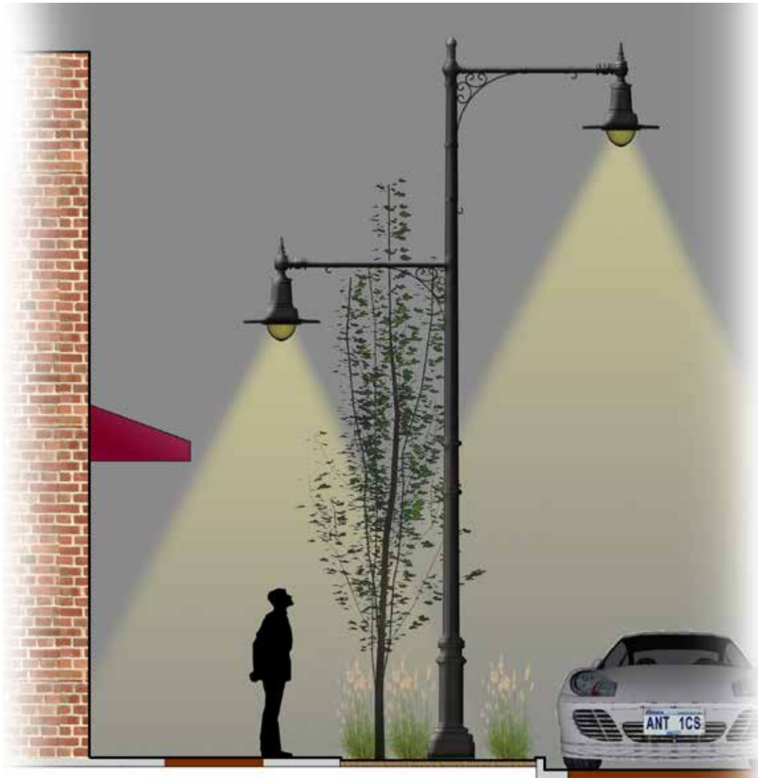
Figure 2.22 The shared light pole is another option to light the Main Street corridor.
