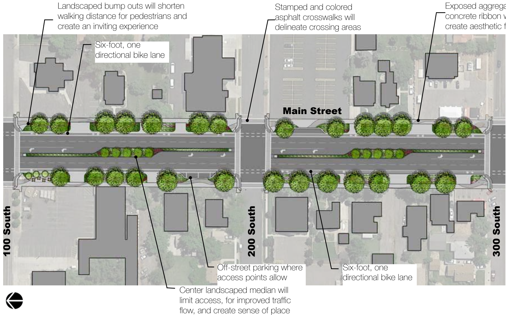
Figure 2.29 The South Transition Area will continue the center median from the Downtown Core, however, the decreased sidewalk width and building setbacks create wider landscape planter beds that can accommodate the existing London Plane trees, if sight lines allow.
