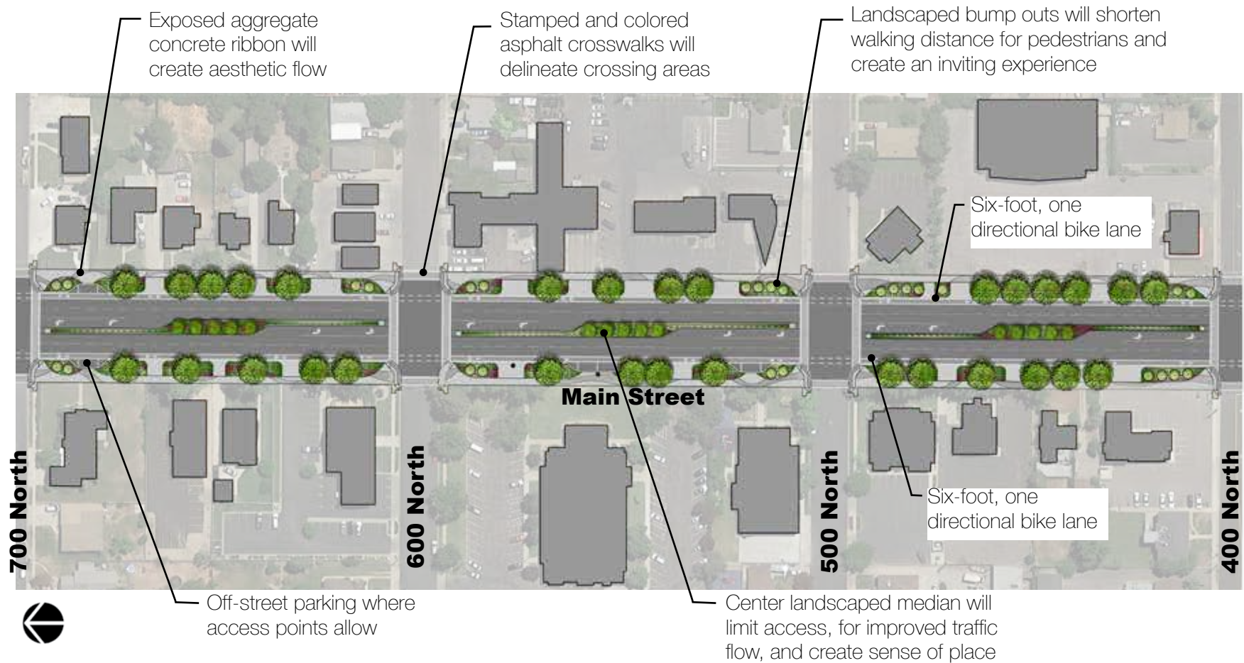
Figure 2.28 The North Transition Area will continue the center median from the Downtown Core, however, the decreased sidewalk width and building setbacks create wider landscape planter beds that can accommodate the existing London Plane trees, if sight lines allow.
